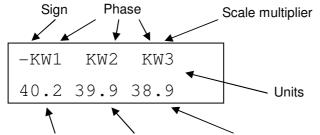
L1 phase measure L2 phase measure L3 phase measure
