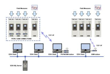
System for measurement and analysis of power quality over distribution networks
